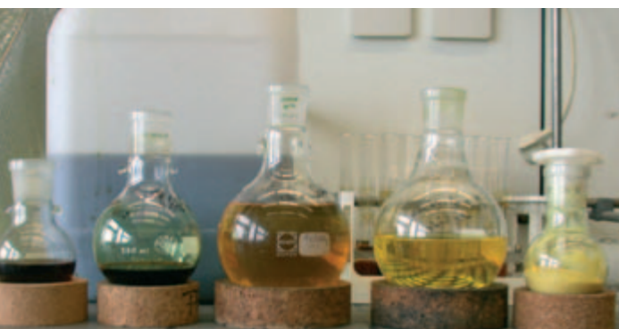
From left to right the crucial extract from the fungus and the different purity steps resulting from the crude extract during the purification process
